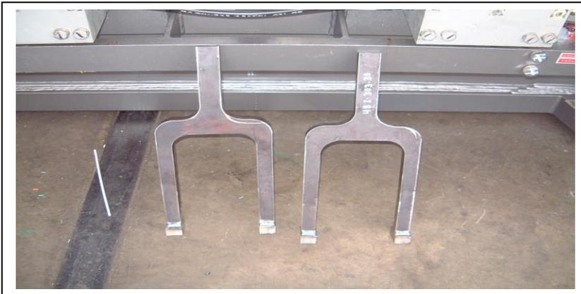
**LOWER STRIPPER BEAM STOPS FOR FLOOR LEVEL MACHINES
