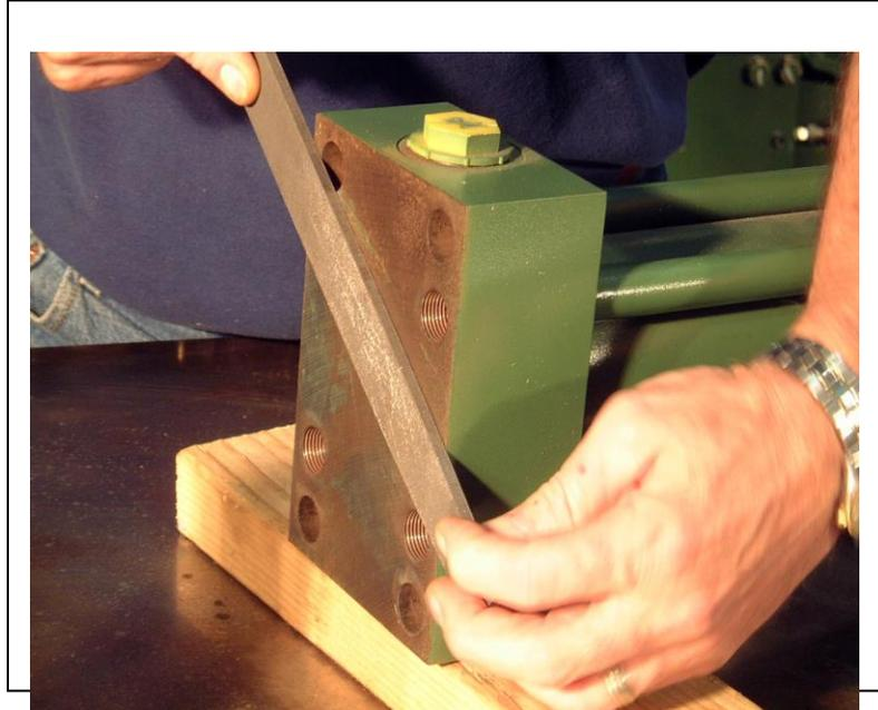
Clean stripper cylinder base with Scotch-Brite or Bear-Tex hand pads. Using a flat fine tooth file remove any scratches or nicks raised areas only.
